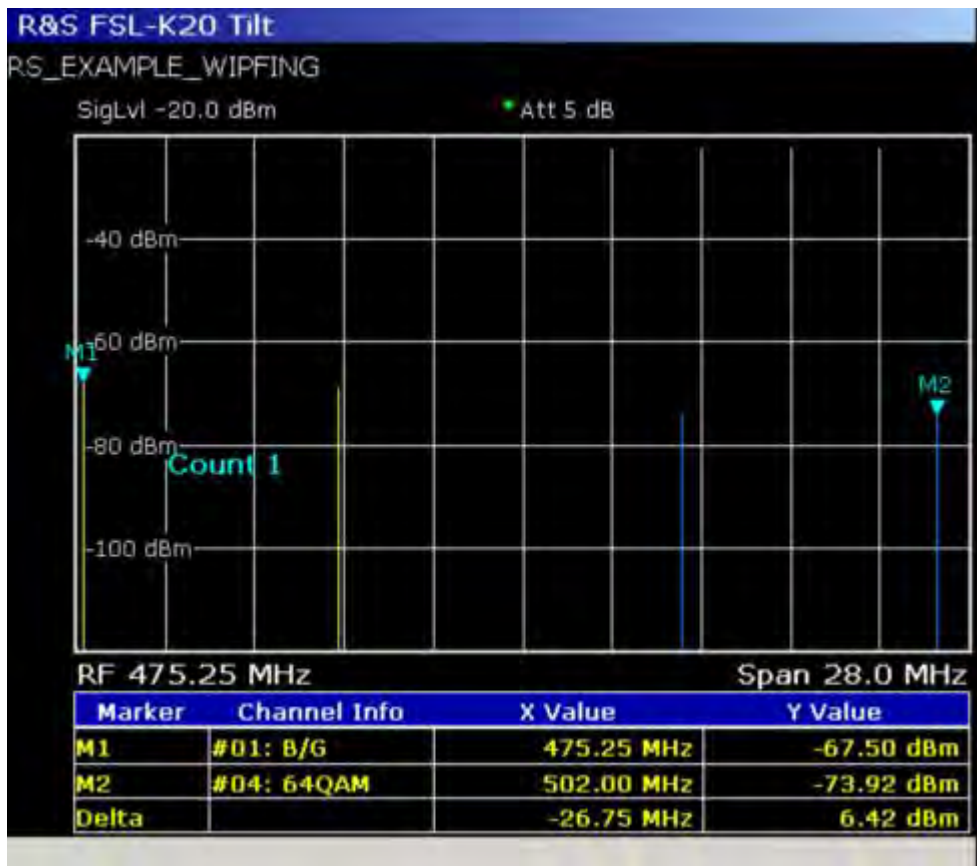
Fig. 2-57 Tilt measurement using a Channel Table. No input signal!
