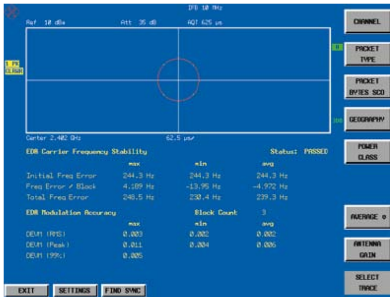
Measurement of initial carrier frequency tolerance of a Bluetooth® signal with R&S®FS-K8.
