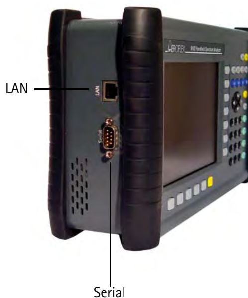
Figure 2 9102 connectors on the left-hand side of the instrument
