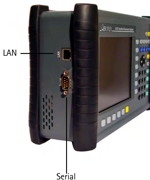
Figure 2 9101 connectors on the left-hand side of the instrument
