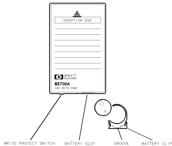
Figure 3-3. Memory card battery replacement.
