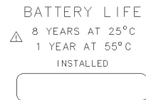
Figure 3-4. Rear-panel battery information label.
