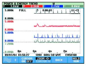
AutoTrend automatically records all displayed parameters in the background. Toggle between data and trend view and use cursors and zoom to analyze measurements without interrupting the recording.
