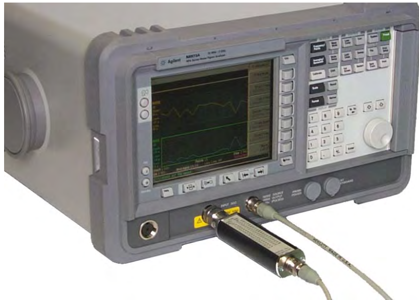
Figure 1-1 NFA with a Normal Noise Source connected
