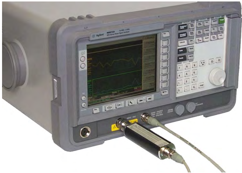
Figure 1-1 NFA with a Normal Noise Source connected
