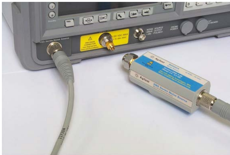
Figure 1-5 Operator's Check Test Setup for Data Communication
