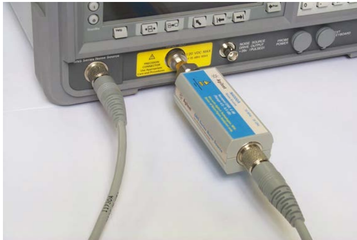
Figure 1-12 SNS connected to NFA graphic
