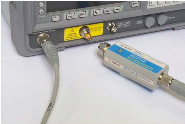
Figure 1-8 Operator's Check Test Setup for T_{\text{cold}} Communication
