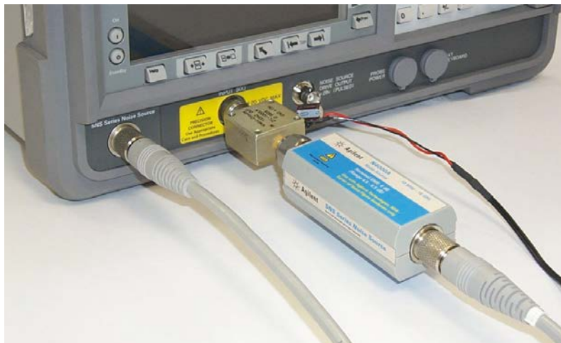
Figure 1-4 Typical Noise Figure Measurement Test Setup
