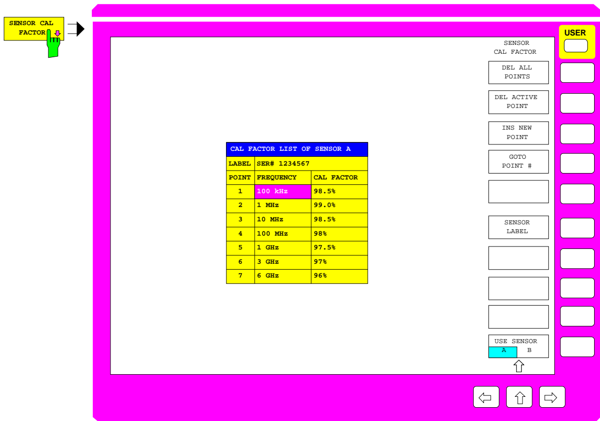
Fig. 2-42 Entry of a frequency-dependent calibration factor
