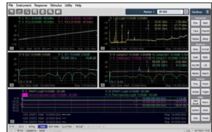
In addition to S-parameters, the spectrum analysis, gain compression, and differential I/Q applications are used to characterize a 10 MHz to 125 GHz amplifier.
