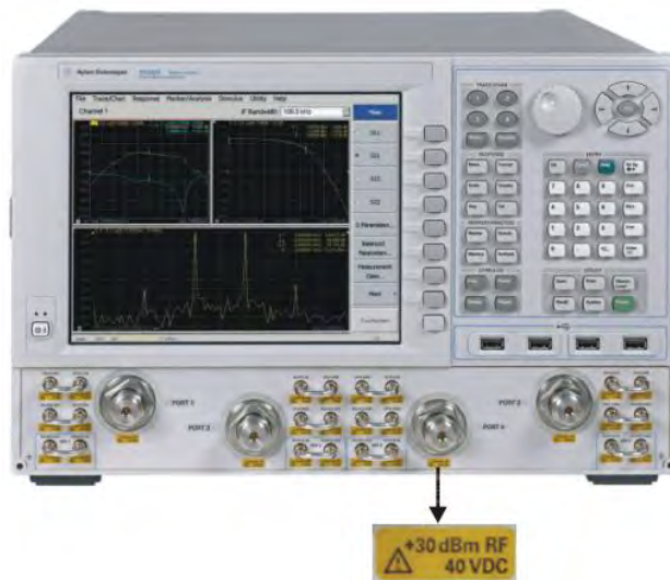
Figure 2. Example Label Showing Damage Level for Each Port and Connector
