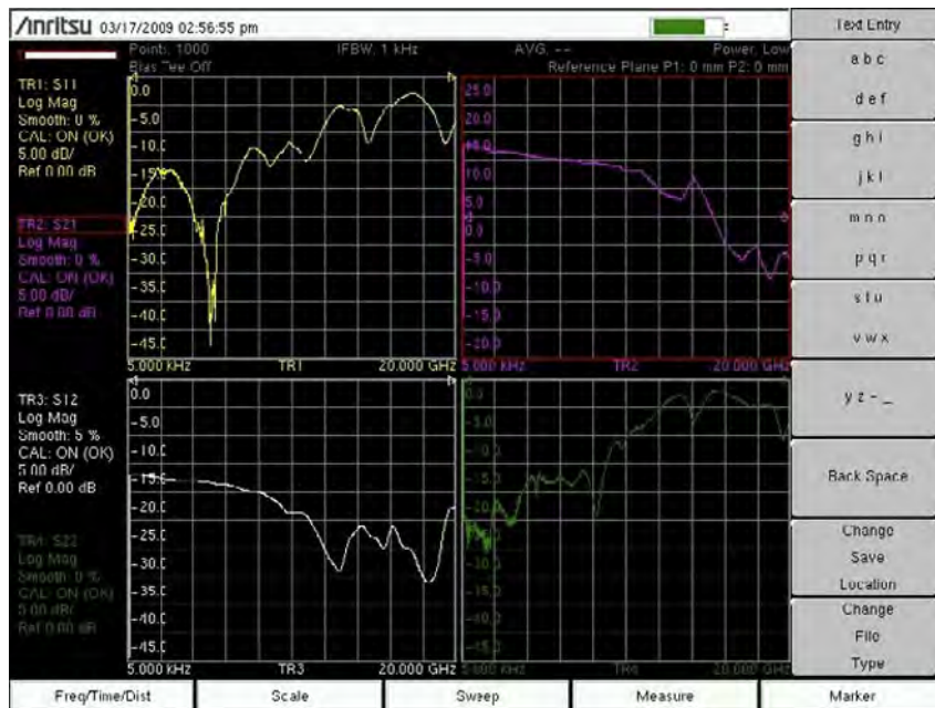
Figure 5-8. Gain, Input Match, Output Match, Isolation of an Amplifier
