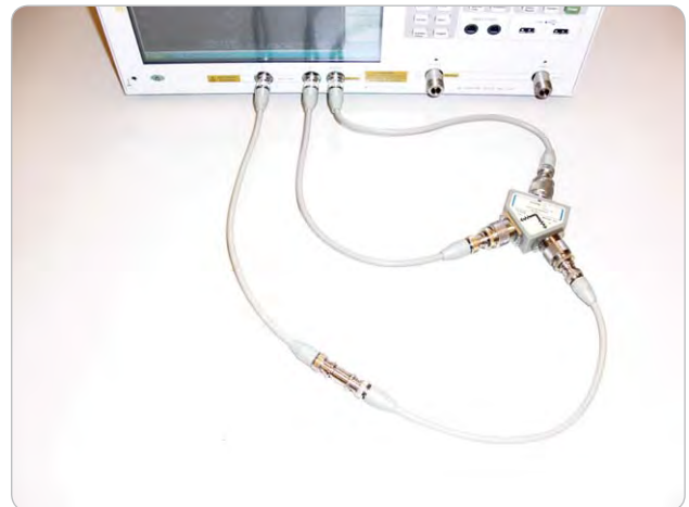
11667A and E5061B: 8120-1838 cables and 1250-0780 adapters are used (refer to page 5.)
