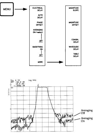
CENTER 32.265975000 GHz SPAN 15.0000000000 GHz Probably the most frequently used feature to improve the data presentation is averaging. Press RESPONSE (MENU), then [AVERAGING ON/restart]. The active function is now the averaging factor applied to the measurement.
