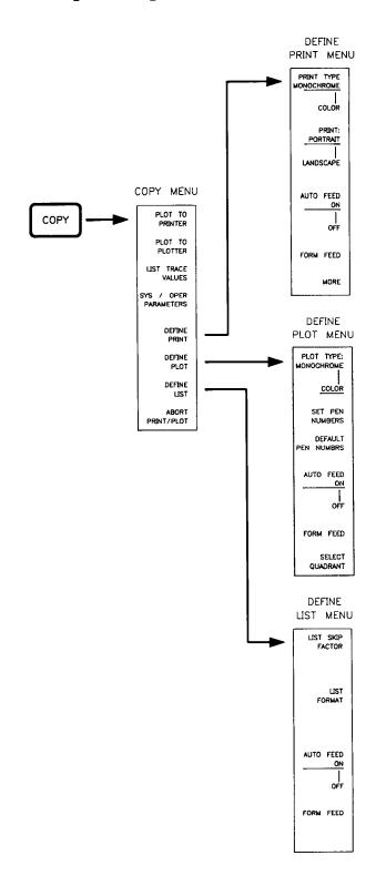
Measurement results can be output to a graphics printer, digital plotter, or a line printer using using selections in the <u>COPY</u> menu structure. The HP 8510C adds two RS-232 ports for connection of hardcopy output devices. Moving the output devices from the 8510 system bus to the RS-232 ports may improve measurement throughput because since the RS-232 ports are fully buffered, the measurement can continue while the plot is being produced.
