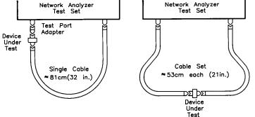
The point(s) at which the device under test is connected to the test set is called the Reference Plane(s). If cables are used to extend the test set port out to the device under test, the end of the cable is defined as the Port 1 and Port 2 reference plane. All measurements are made with respect to the reference plane(s).
