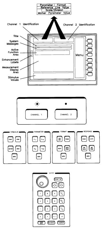
**CRT Display.** The front panel of the network analyzer is relatively simple. It is shown in full by the foldout at the end of this document. First, there is the CRT which presents the measurement results. This illustration shows the general areas for the measurement trace and for the various annotations which communicate to the operator.
