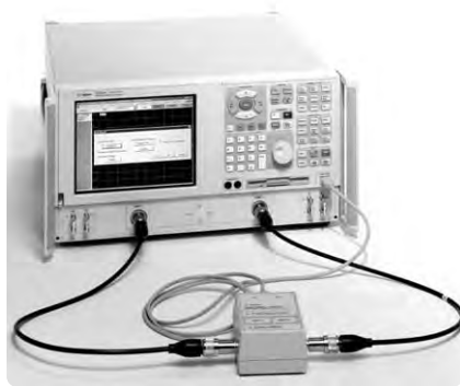
Calibration configuration using the PNA series
