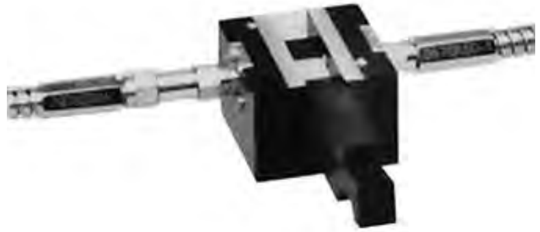
Figure 8-21. Active Device Test Fixture
