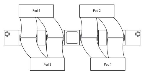
In a multi-card set, pods are indexed from the bottom up. Because clock signals can be input to any card in the set (on pod 1 or 3), cards do not have *master* and *expander* designations.
