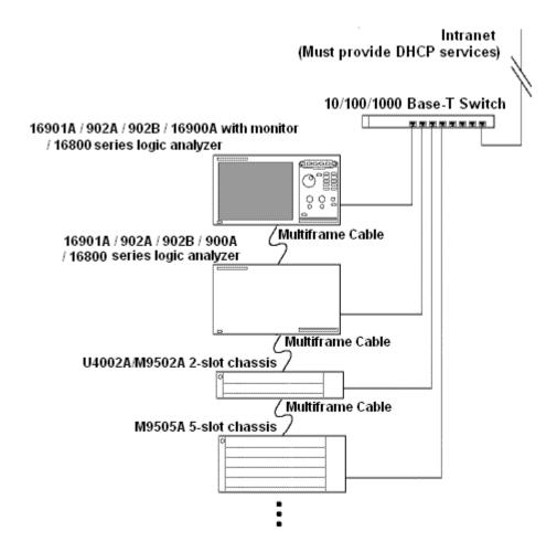
In the simple multiframe configuration using an Intranet, all of the systems are connected to the common network using their LAN port.
