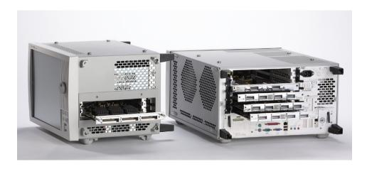
The Agilent Technologies 16900 Series logic analysis systems are modular systems with slots for logic analyzer and other types of measurement modules.
