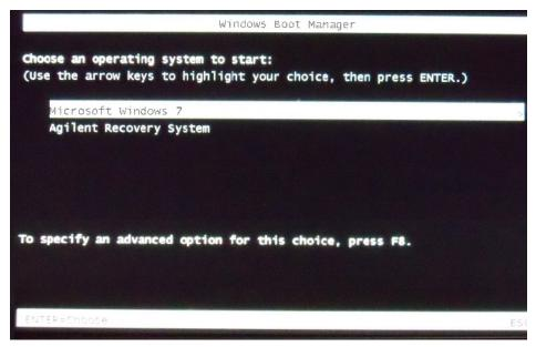
2 After a few seconds, the Logic Analysis system automatically starts with the option selected in the Windows Boot Manager. Select the **Agilent Recovery system** option in the Windows Boot Manager screen using the arrow keys and then press Enter.
