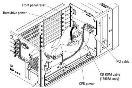
**4** Remove screws from the back of the CPU tray using a Torx T-10 screwdriver.
