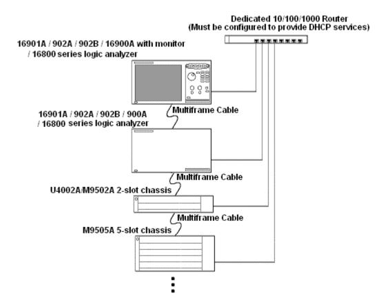
In the simple multiframe configuration using an isolated router, all the systems are connected to the common network using their LAN port.
