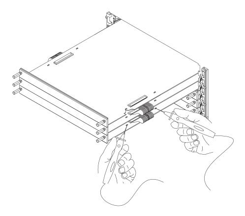
If there is continuity (0 ohms), the flex cable is seated correctly in the connector.
