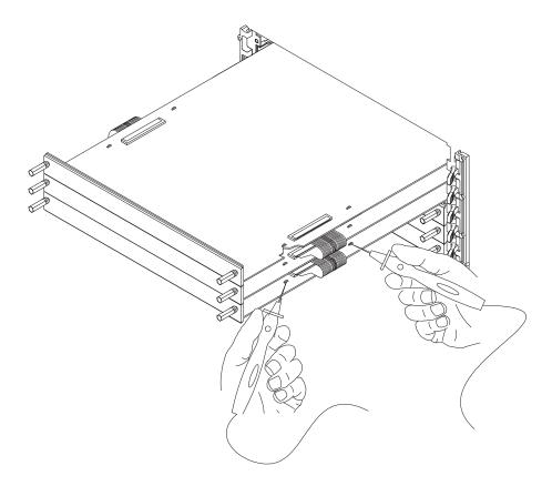
If there is continuity (0 ohms), the flex cable is seated correctly in the connector.
