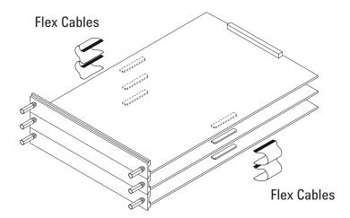
**1** Insert the lowest card about 1/3 of the way into the desired logic analyzer frame slot.
