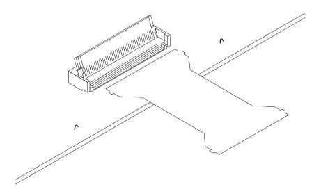
**b** Place the flex cable into the connector, exposed conductive traces towards the card, so that the flex cable ears are secured by the connector guides.
