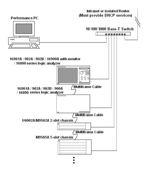
In the performance multiframe configuration, you run the *Agilent Logic Analyzer* application on a high-performance PC or server. This is useful if you are trying to maximize multiframe logic analysis system performance.
