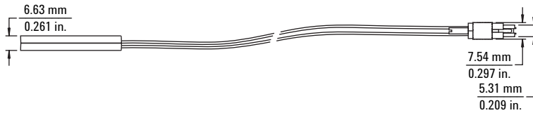
Figure 3.6. E5394A and E5396A soft touch probe dimensions
