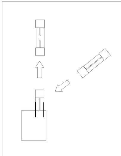
To check or replace the fuse, pull the fuse holder and remove the fuse. To reinstall the fuse, insert a fuse with the proper rating into the fuse holder.
