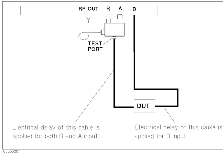
**Figure 8-16. Port Extension With the T/R Test Set**
