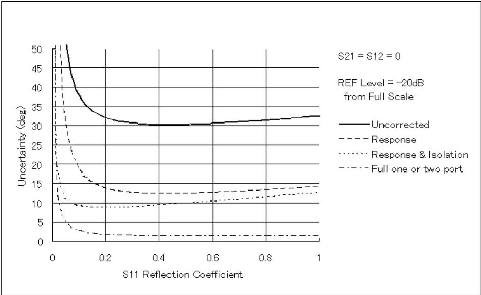
Figure 11-16. Total Reflection Phase Uncertainty of One-Port Device
