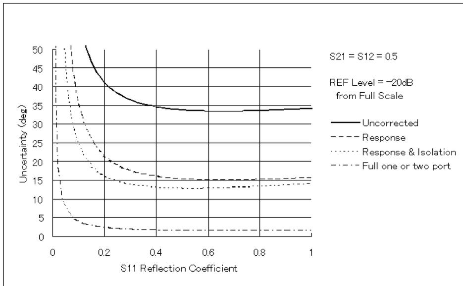
Figure 11-18. Total Reflection Phase Uncertainty of Two-Port Device
