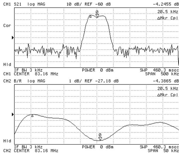
Figure 10-4. Using Peak Search to Determine Ripple
