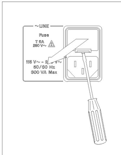
Lever a small minus screwdriver to dismount the fuse holder above the AC line receptacle on the rear panel.
