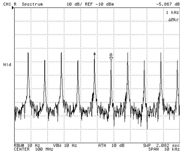
Figure 10-20. Zooming Carrier Signal of FM Signal
