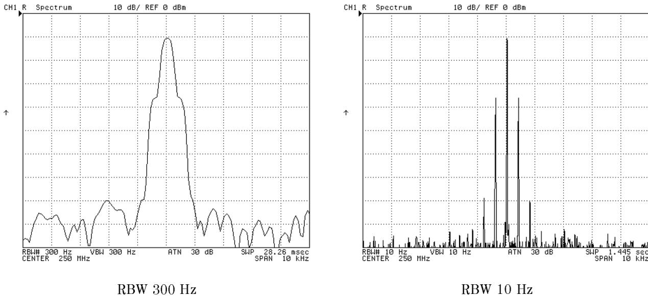
Figure 6-16. Setting Resolution Bandwidth (RBW)
