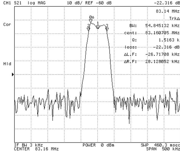
Figure 10-3. Using the Marker to Determine 6 dB Bandwidth
