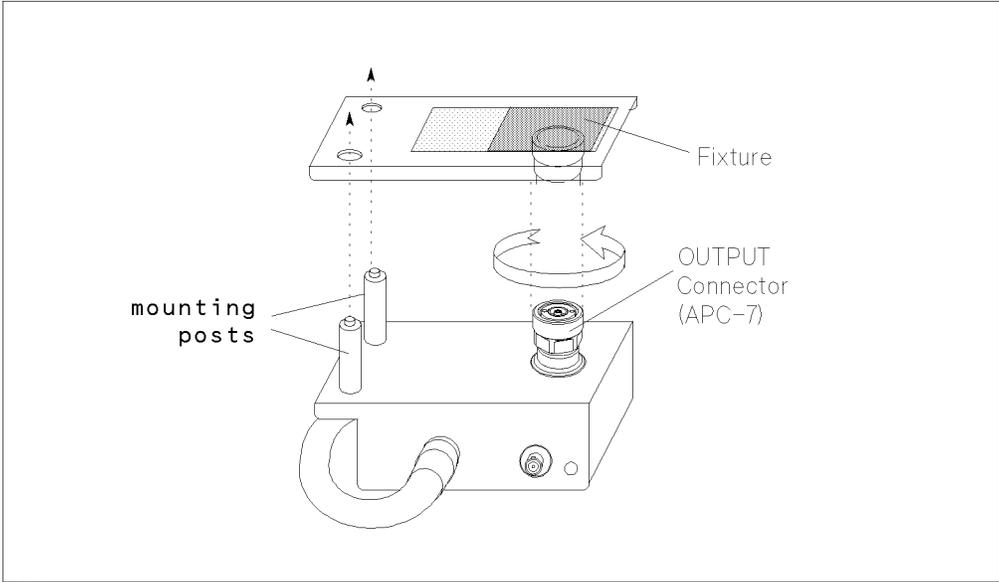
**Figure 7-2. Connecting Test Fixture**
