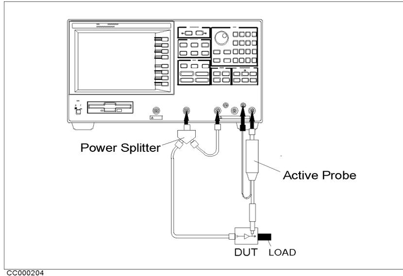
**Figure 2-6. Network Analyzer Mode (One Active Probe)**
