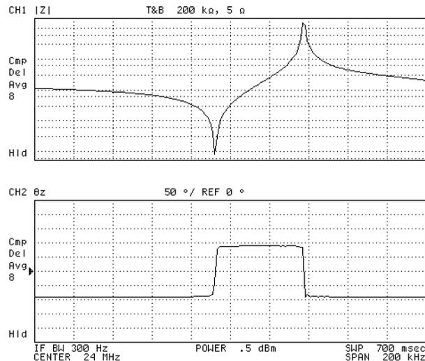
Figure 10-27. Frequency-based Characteristics of a Crystal Resonator
