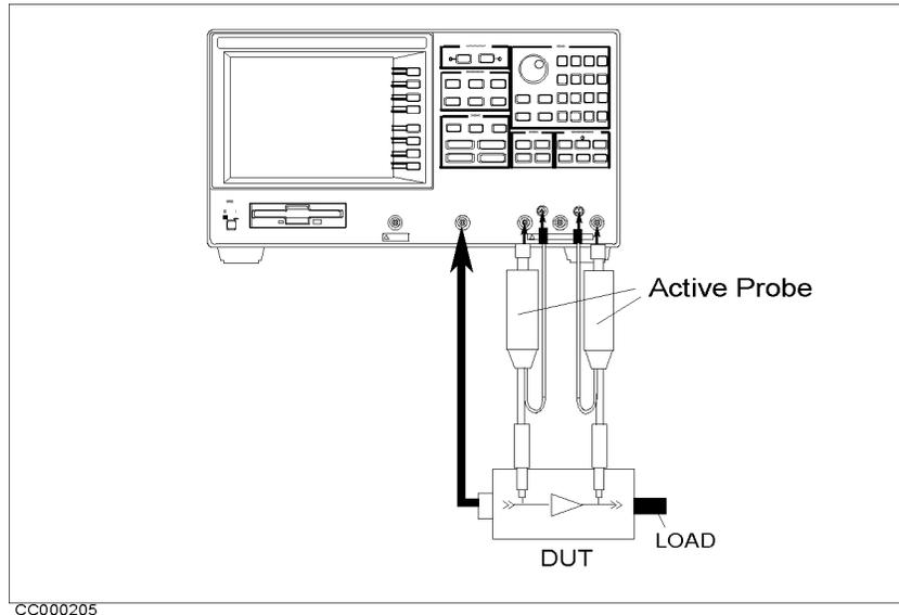
**Figure 2-7. Network Analyzer Mode (Two Active Probes)**
