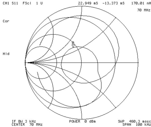
**Figure 10-13. Admittance Measurement**
