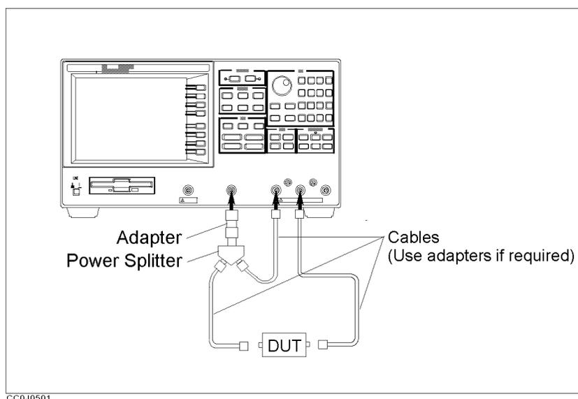
Figure 5-1. Connecting DUT for Directional Transmission Characteristic Measurement
