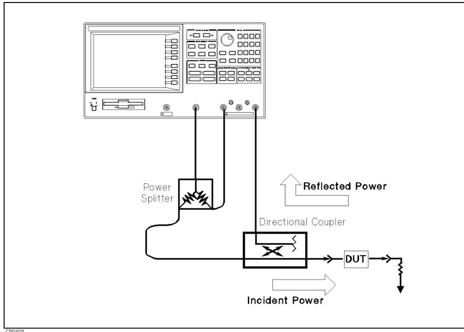
Figure 10-7. Reflection Measurement
