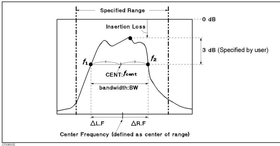
Figure 8-12. Parameters of a Band Pass Filter Measurement
