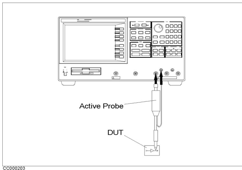
**Figure 2-5. Spectrum Analyzer Mode (One Active Probe)**
