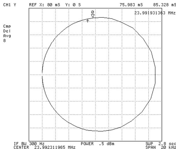
Figure 10-31. Admittance Chart for a Crystal Resonator
