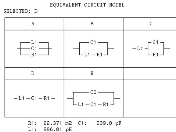
Figure 10-25. Equivalent Circuit Parameters
