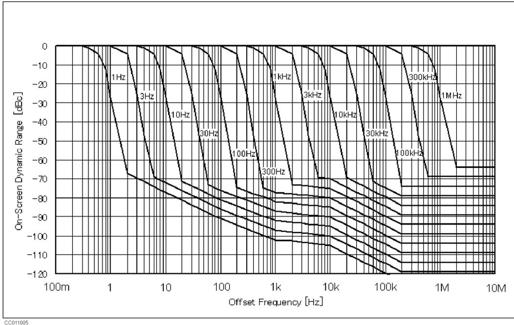
Figure 11-5. Typical On-screen Dynamic Range (Center: 50 MHz)
