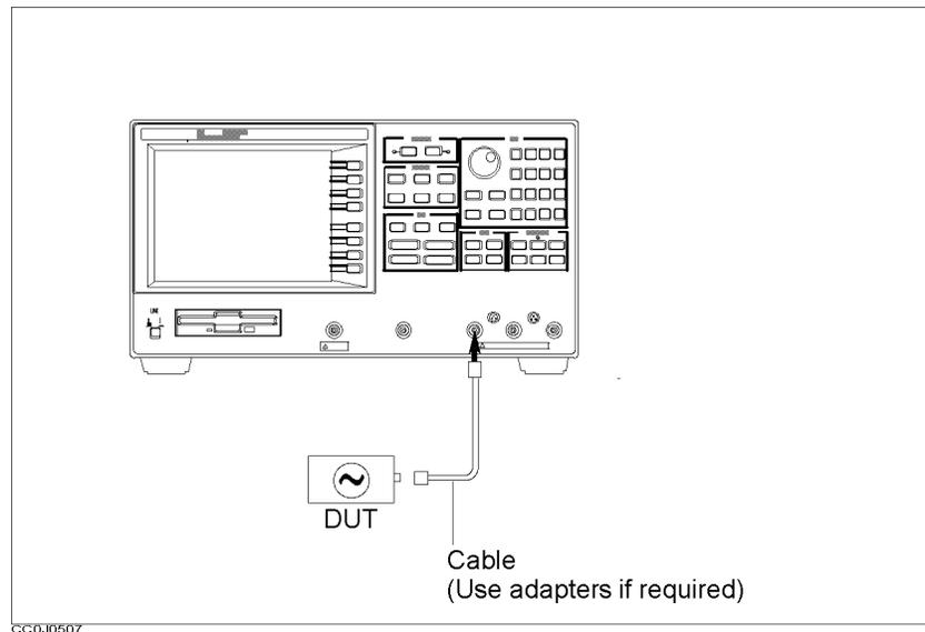
**Figure 5-7. Connecting DUT When Directly Measuring the Signal**
