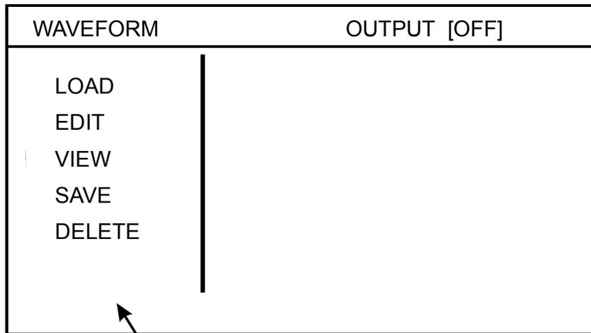
— Selecting VIEW will display the waveform in the scratchpad as shown below.
