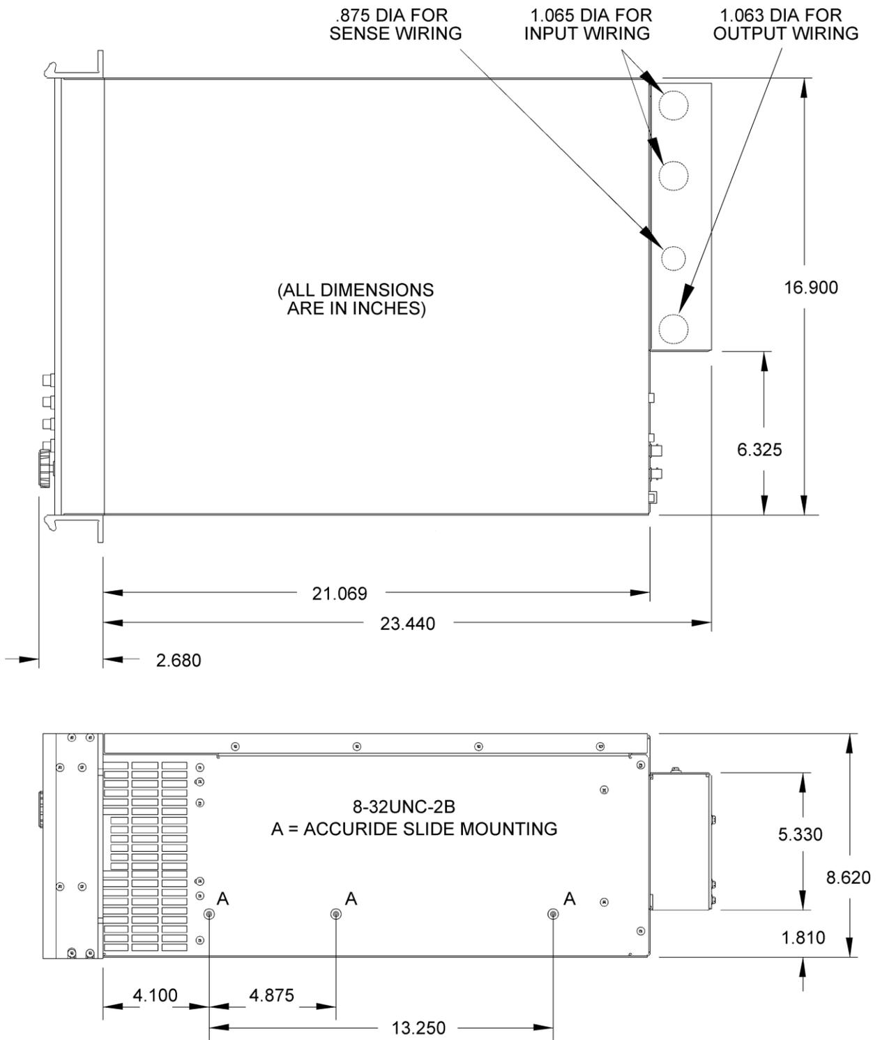
**Figure 2-2 Mounting Dimensions, SmartWave Top and Side Views**
