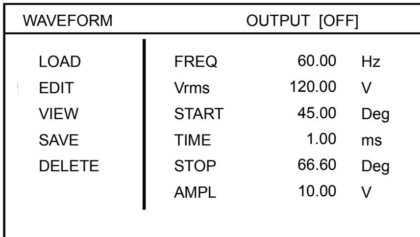
9. Select **Vrms**. Enter **120**, then press **<Enter>** to set the RMS voltage to 120 volts.
