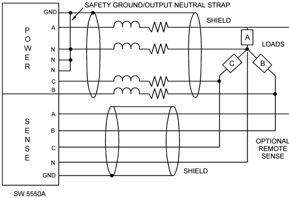
**Figure 2-5 Sense Lead Connections for 3-Phase Output**
