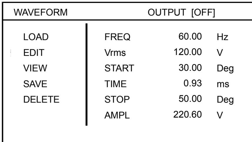
9. Select **Vrms**. Enter **150** using the keypad, then press **<Enter>** to set the RMS voltage to 150 volts.
