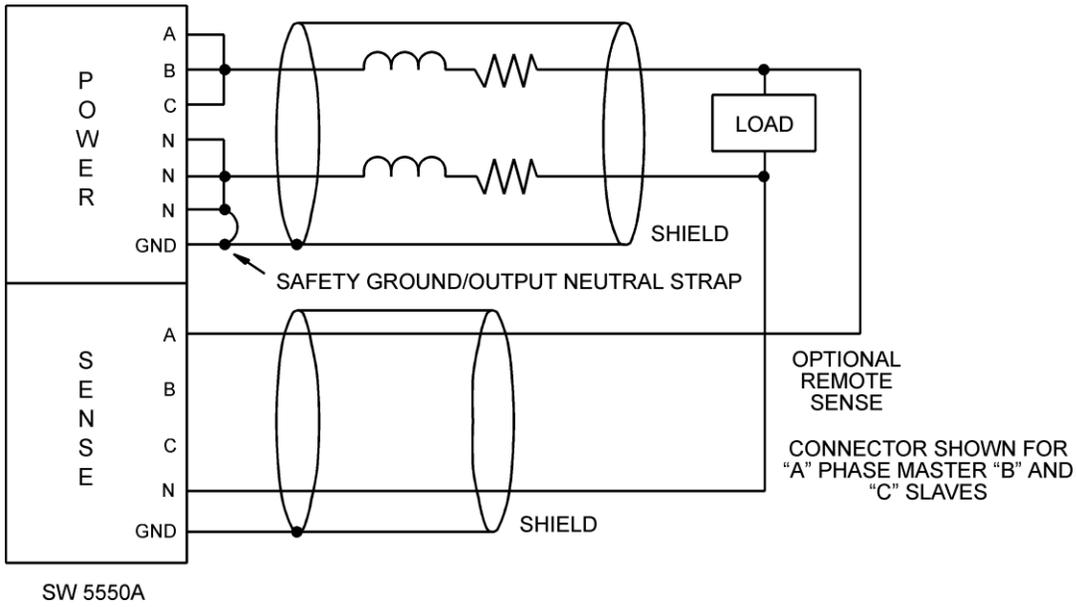
**Figure 2-4 Parallel Connections**
