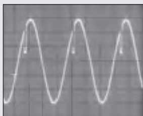
Sine wave with a dropout from 45° - 60°
